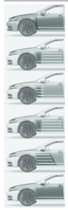
Adjacent panel: sand panel with suitable abrasive e.g. Trizact - P1000 New part / repair: sand surfacer (minimum P500)
